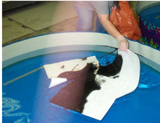
Figure 6. Sorbent pads used in calm conditions
