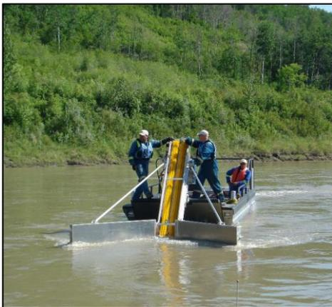
In 2007 WCSS purchased the advancing Bow Skimmer, designed to be mounted on one of the barges and used for the collection of hydrocarbon, oil emulsions and oily debris in relatively calm conditions. It has been deployed twice to be used in spill response since 2007.
